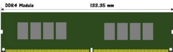
284 pin, 0.85 mm pitch, 1:1 Signal/Ground ratio
