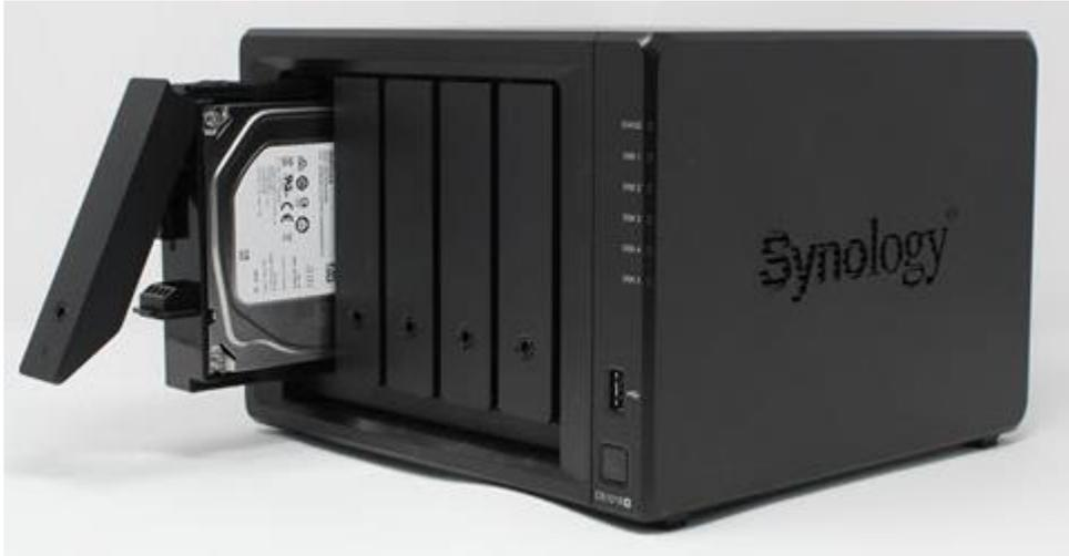
A NAS can have multiple bays (2,4,6,8 common) containing high capacity disk drives.
