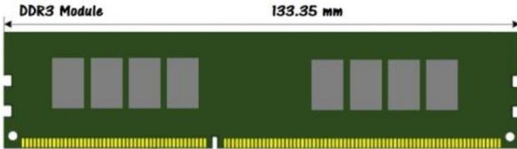
240 pin, 1.0 mm pitch, 2:1 Signal/Ground ratio
